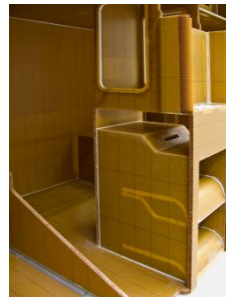
Detail of an assembly for aircraft interiors (complete base structure done by EC)
