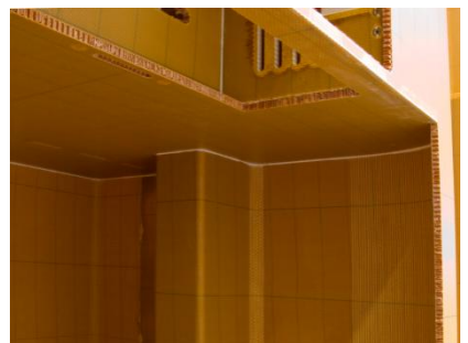
Detail of an assembly for aircraft interiors (complete base structure done by EC)
