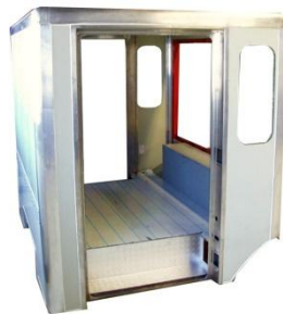
Production and assembly of a cabin for a fire engine
