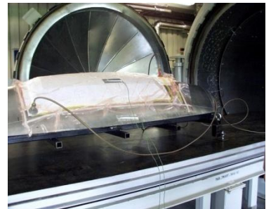
Part prepared for autoclave process
