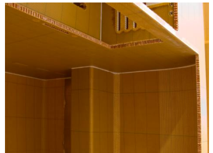
Detail of an assembly for aircraft interiors (complete base structure done by EC)
