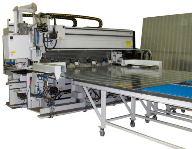
FSW unit during production of a large format panel
